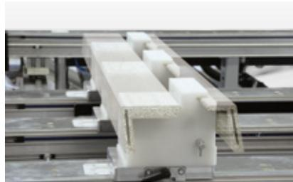
Clamping fixture for facings: Vacuum clamping fixture for a pair comprising rebate and ornamental facings according to customer design. Mounted on a base plate module.
