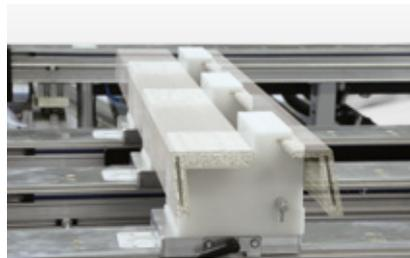
Clamping fixture for facings: Vacuum clamping fixture for a pair comprising rebate and ornamental facings according to customer design. Mounted on a base plate module.
