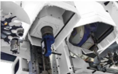
**Rapid tool change:** As it is designed with two trimming spindles, the chip-to-chip times are reduced and productivity is increased. While one spindle mills, the second inserts the tool for the next processing step.
