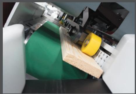
▶ Integrated acceleration belt with driven fence for quick and exact positioning of workpieces that exit the saw.
