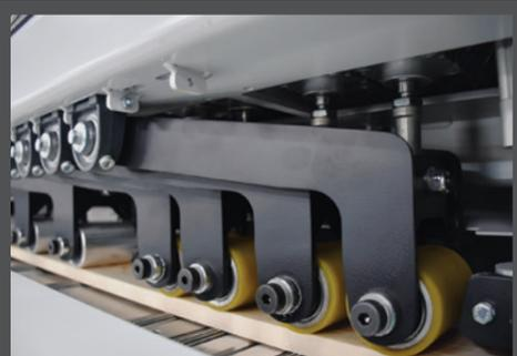
▶ Heavy-duty infeed design featuring 9 driven bottom rollers and 9 top rollers. The rollers are supported on both sides to maximize and surface contact to each workpiece to provide excellent cut precision.
