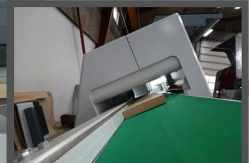
► The 30° angle design of the saw allows correct workpiece positioning during cross-cutting. Due to gravity along the 30° incline, waste and defect material can be removed with ease.
