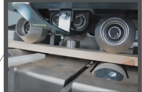
▶ Integrated double top and bottom rollers ensure accurate infeed of workpieces.
