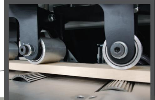
▶ The bottom feed rollers are placed high above the bed plate of the machine. This enables the processing of bent and twisted timber, and results in maximum productivity and cut accuracy.
