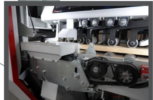
► The high quality, servo-driven timing belt of the bottom rollers ensures accurate cutting. Its design has proven to be extremely durable, requiring only a minimum of maintenance.
