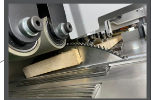
► Maintenance-free, mechanical waste gate ensures optimal and easy removal of small waste and defect pieces inside the saw unit, resulting in precise sorting of workpieces.
