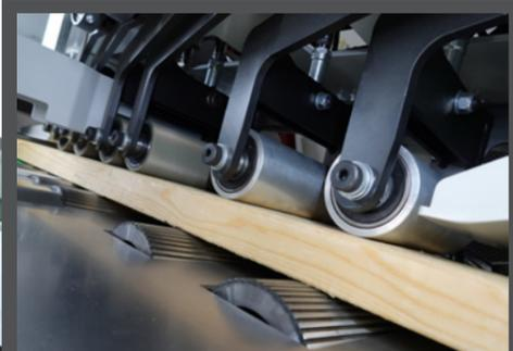
► The bottom feed rollers are placed high above the bed plate of the machine which allows feeding of bent or twisted timber, and ensures maximum productivity and accuracy.
