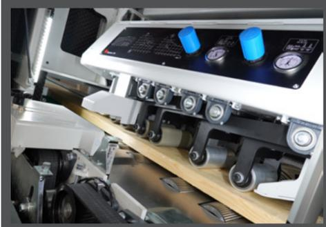
► Heavy-duty design with strong double side supported top pressure rollers. This ensures maximum contact between workpieces and feed roller. Also, it enables reliable cut precision and high acceleration and deceleration.
