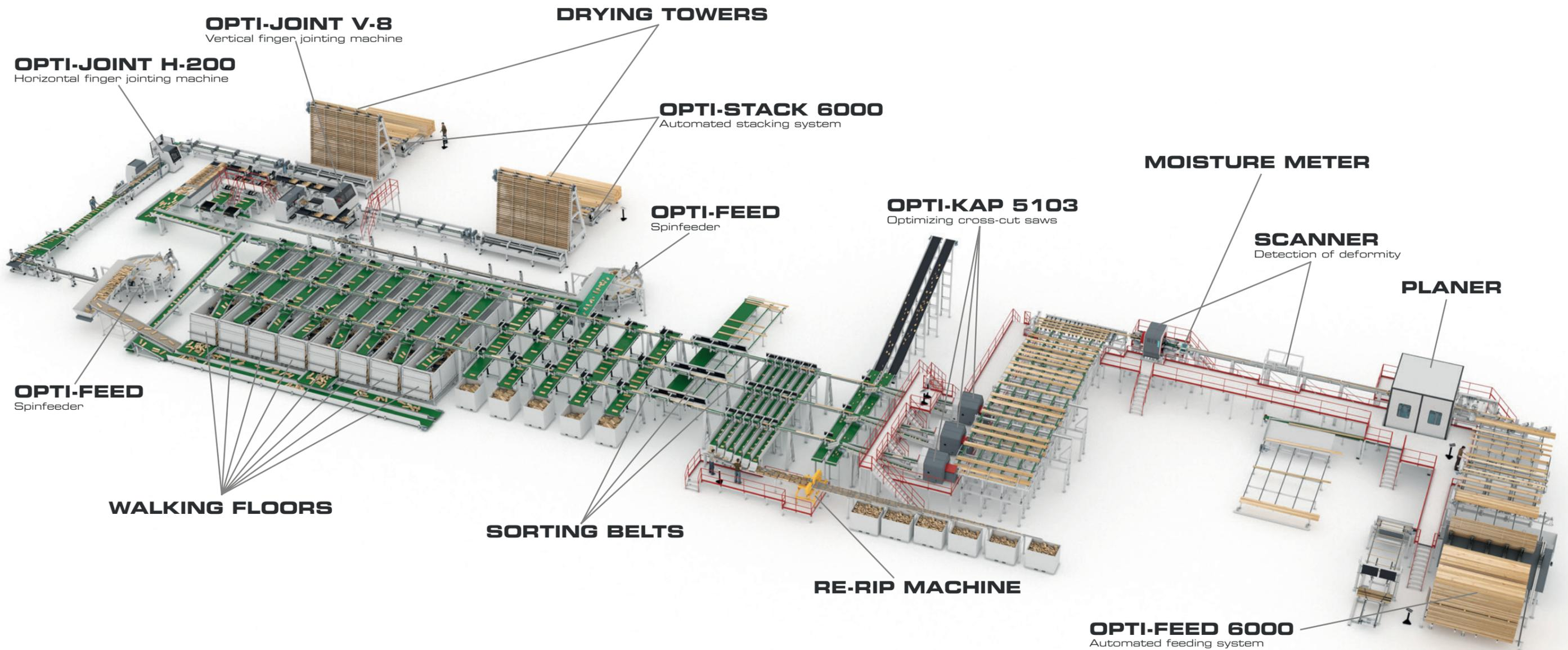
This Opti-Solution is an optimizing cross-cut line that starts with an Opti-Feed 6000 automatic feeding system, followed by a planer, a MiCROTEC Curvescan scanner, and a moisture meter.
