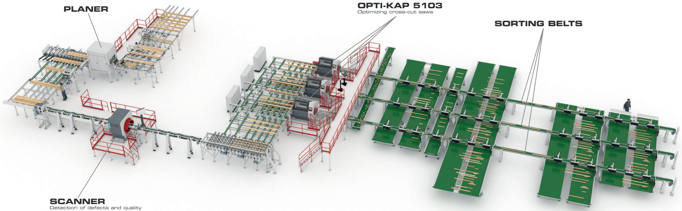
This Opti-Solution is an optimizing cross-cut line featuring an Opti-Feed 6000 feeding system that feeds batches of workpieces to a planer. After the planer, workpieces are automatically transported to a Microtec Goldeneye 502 scanner including X-ray for the detection of defects and quality.
