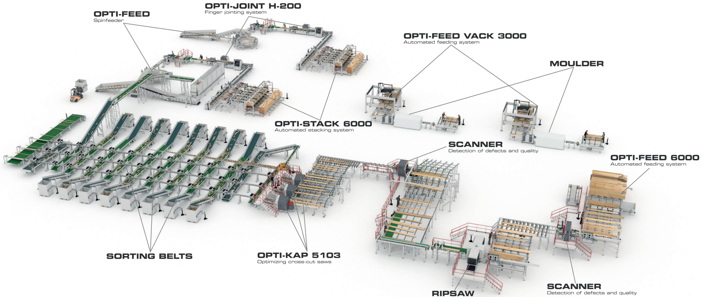
This Opti-Solution is an optimizing cross-cut line that starts with an Opti-Feed 6000 automatic feeding system, followed by a MICROTEC rip scanner and a rip saw.
