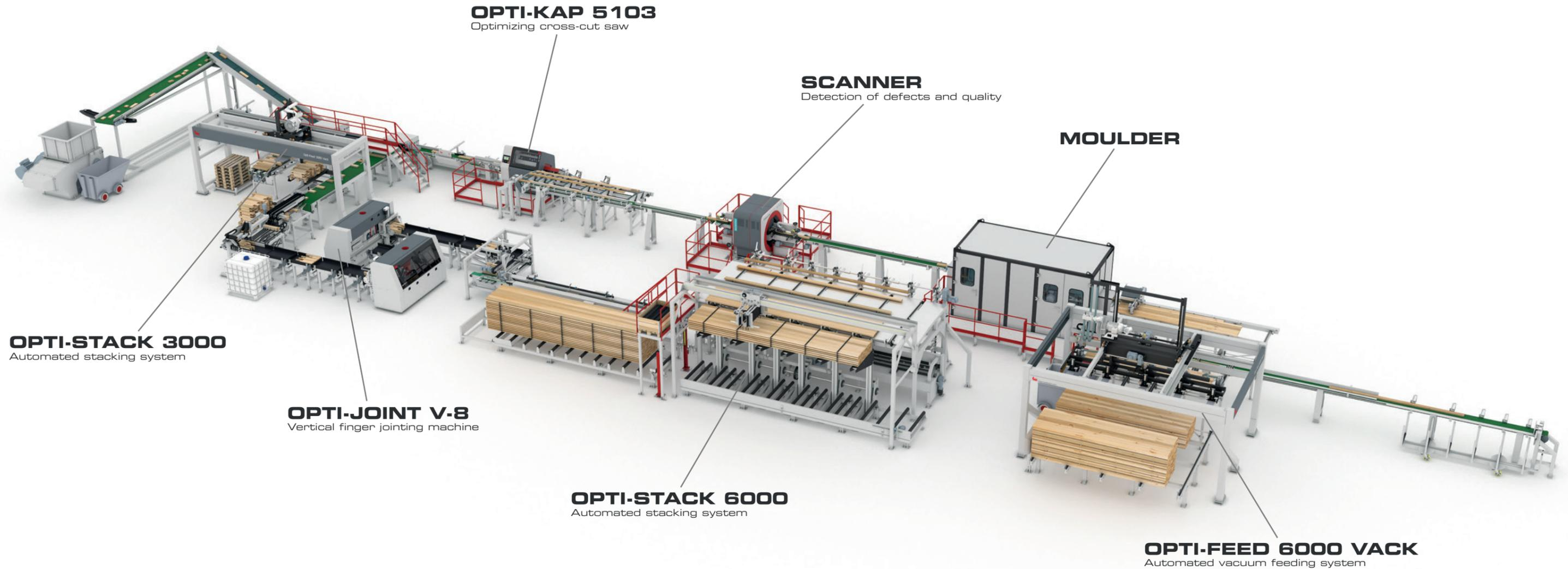
This Opti-Solution is an optimizing cross-cut line that starts with an Opti-Feed 6000 Vack automatic feeding system, followed by a moulder.
