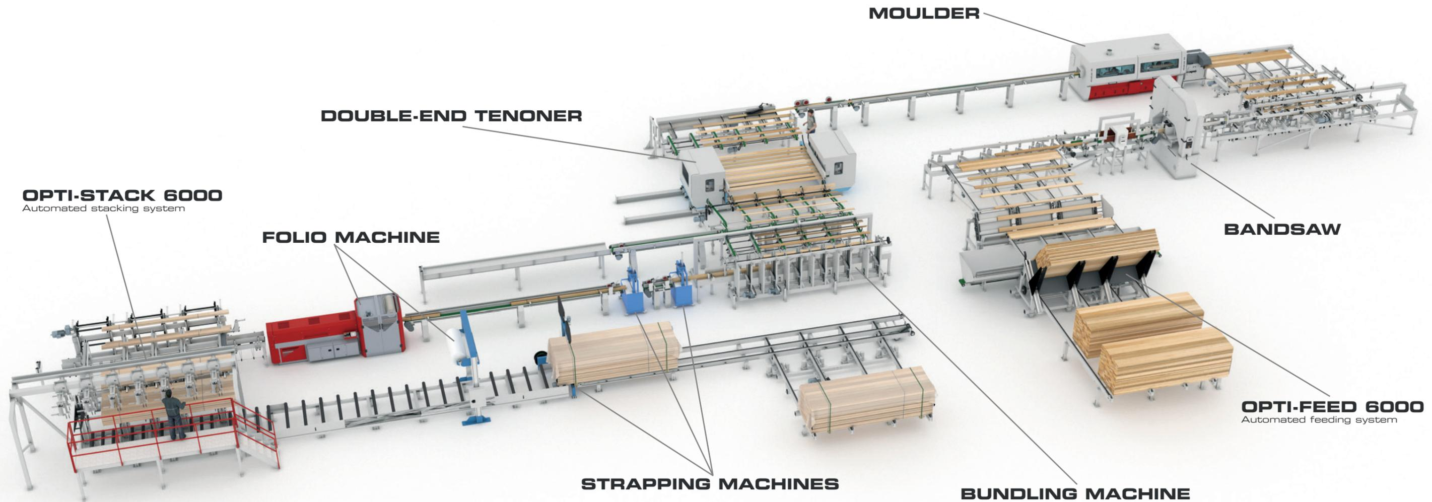
This Opti-Solution is a material handling system featuring an Opti-Feed 6000 automatic infeed system that automatically feeds workpieces into a bandsaw. The bandsaw splits workpieces into two or three pieces, after which workpieces are separated into individual pieces and orientated in the correct order before entering a moulder.
