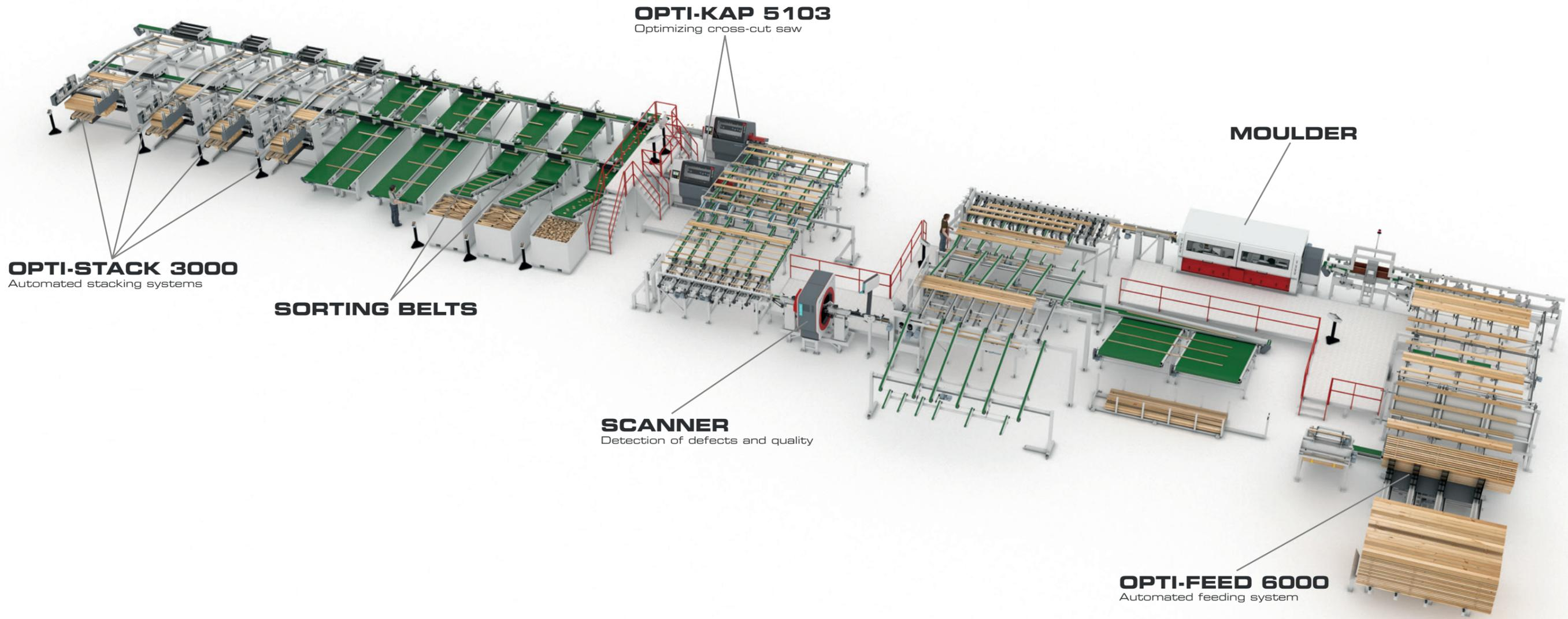
This Opti-Solution is an optimizing cross-cut line featuring an Opti-Feed 6000 automatic feeding system. This automatic infeed system feeds raw material into a moulding machine, in which workpieces are split into lamellas. After the moulder, lamellas are automatically separated into individual pieces and transported to a Microtec Goldeneye 501 scanner that detects defects and qualities.
