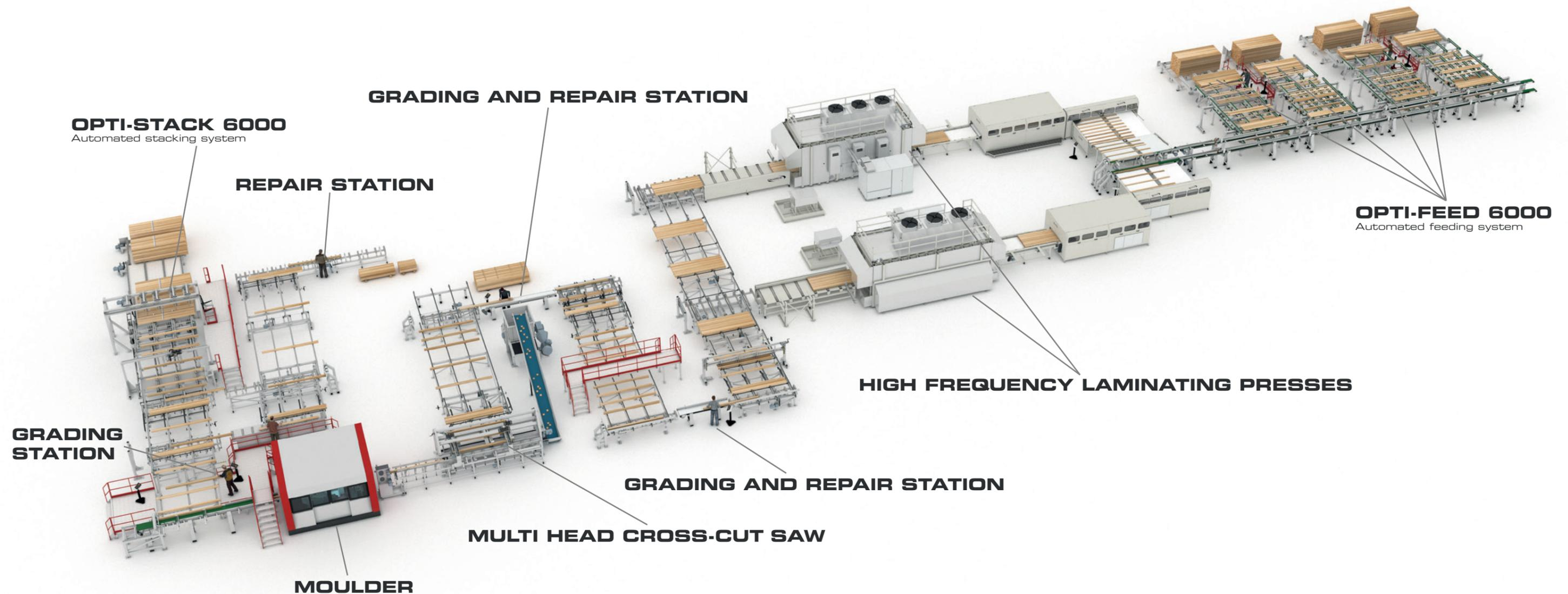
This Opti-Solution is a material handling system featuring four Opti-Feed 6000 feeding systems that feed four different qualities into two high frequency laminating presses.
