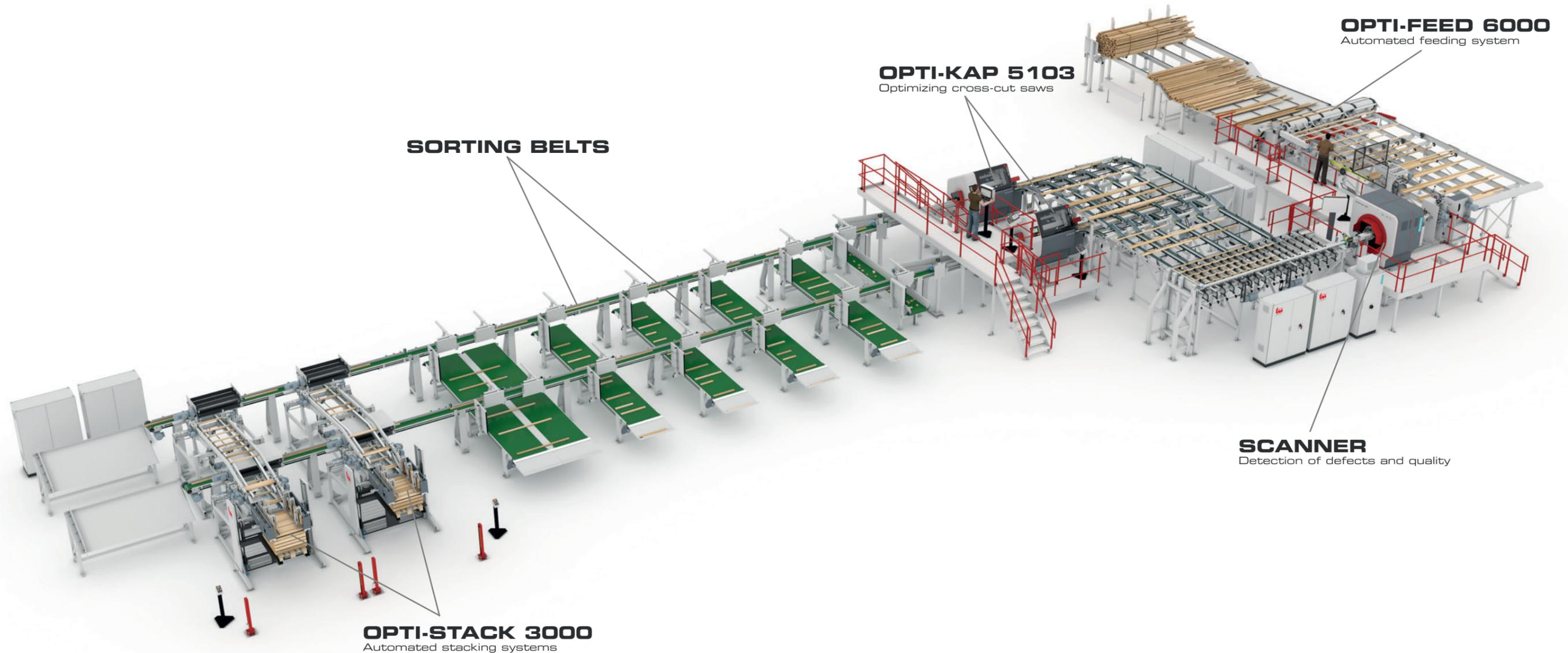
This Opti-Solution is an optimizing cross-cut line that starts with an Opti-Feed 6000 automatic feeding system.
