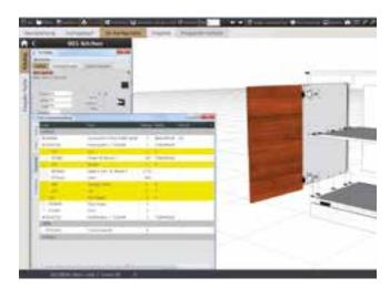
Automatic: BOM resolution. Parts lists are automatically generated at the end of the order processing and are sent to the production system. For the following processes, e.g. for materials management, the data can also be transferred to an ERP system.
