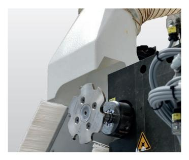
Optimised extraction local to the position of machining larger cross sections
