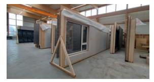
**Before:** The wall units are temporarily fixed to the room in a freestanding position. The assembly of the wall elements and the exact alignment for the window installation takes a lot of time and effort.
