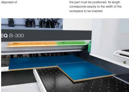
As soon as the LED strip at any point along the cutting line lights up green, the operator knows that there is a finished part that is ready for destacking.
