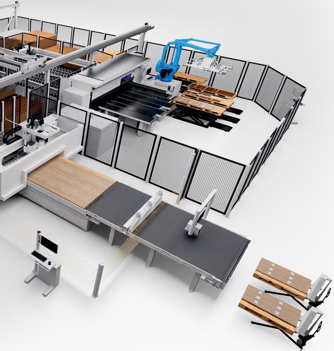
**Combination: storage and saw.** Standardized interfaces enable panel saws to be easily integrated in storage systems and instantly bring noticeable results as a production cell. The storage system puts panels into or removes them from storage quickly, fully automatically and accurately, picks them or transports them to the connected saw. The storage-saw combinations cover the logistical requirements – from woodworking shop customers through to industrial furniture makers.
