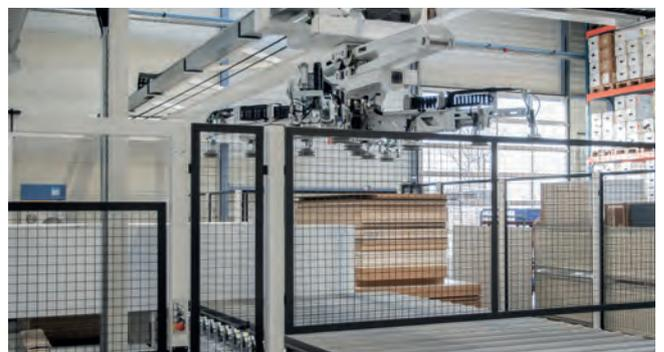
**Processing machines are connected** via standardized interfaces. Regardless of whether you're placing a panel directly on the saw or connecting a processing machine to the storage system using a roller conveyor, the STORETEQ P-300 ensures the connected machines add value optimally.
