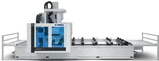
**CENTATEQ P/E-310 – sliding gantry processing centers with five-axis technology and optional edge processing.**
