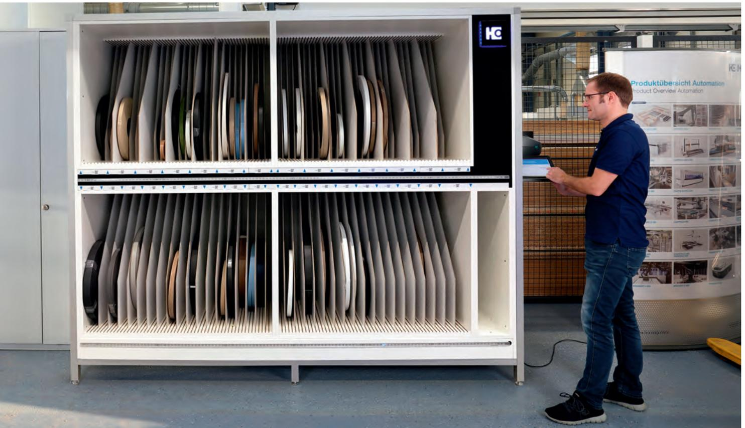
The edgeband assistant helps you to keep a complete overview of all information about your edge material and your material inventory. You can find the right edgeband quickly and easily at any time, eliminating the search for the right material.
