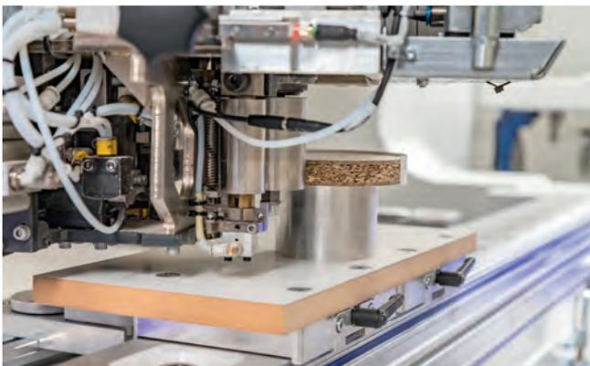
**Precise positioning:** Precise tracing and a feed roller with direct distance measurement guarantee CNC-accurate edge transport. This opens up new possibilities in the design of the shapes and allows perfect results for 360° gluing.
