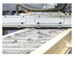
**Automatic calculation of the filling quantity** enables the consistent density distribution of the insulation material.
