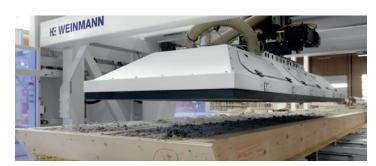
**Rotatable insulation plate at 90°** for automated insulation of roof and ceiling elements.
