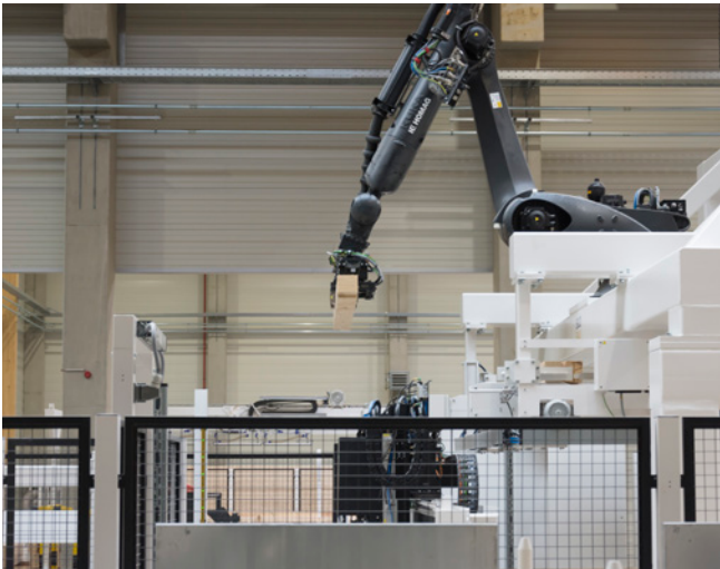
Short cycle times: The robot inserts the wood into the frame work at a speed of up to six cycles per minute.
