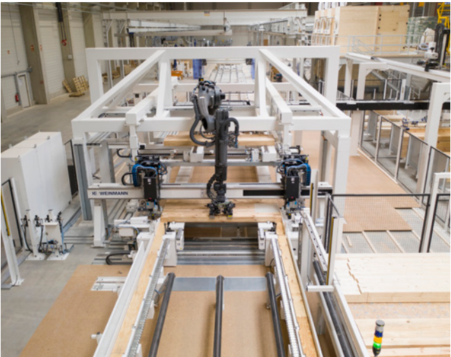
High production flexibility: Depending on the element, the studs are inserted crosswise, longitudinally or diagonally.
