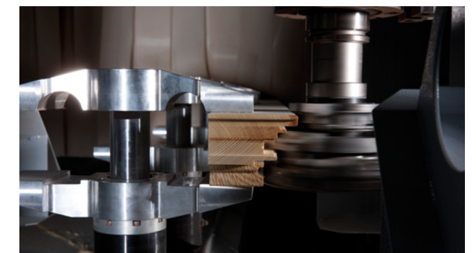
Liquid-cooled trimming spindles with vector control
