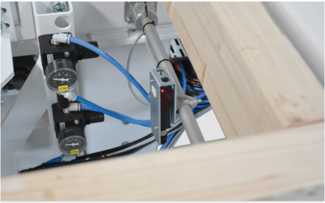
AUTOMATIC ELEMENT DETECTION AT THE X STOP The infeed transport is slowed down, ensuring that the element is not damaged during the operation.
