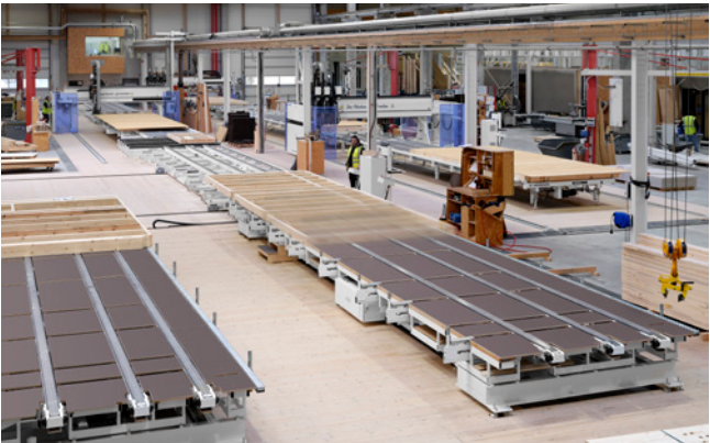
MOTORIZED ELEMENT TRANSPORT Three hinged slat conveyors and roller conveyors on the bottom plate.
