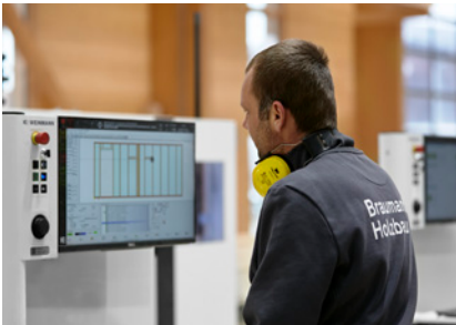
Via wupWorks 3 The CAD data is converted fully automatically and transferred to the machine.
