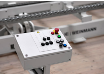
Local control panel With complete control system.
