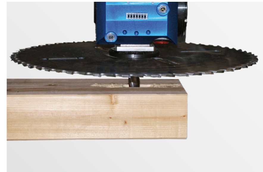
Saw blade with integrated trimming chuck
