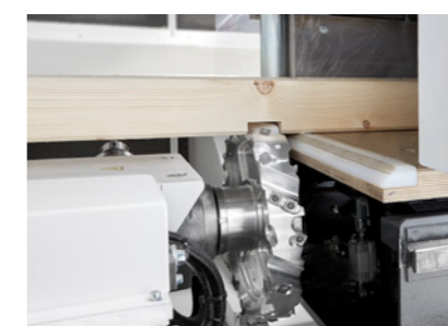
Lap joint with side milling cutter
