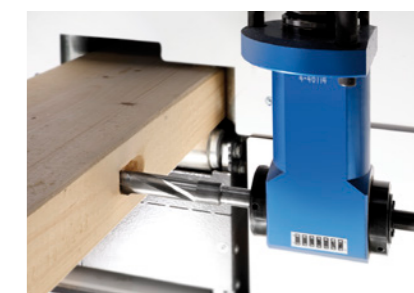
Manufacturing of mortises and pockets
