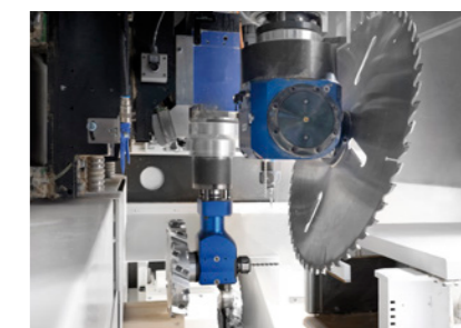
Second integrated main spindle
