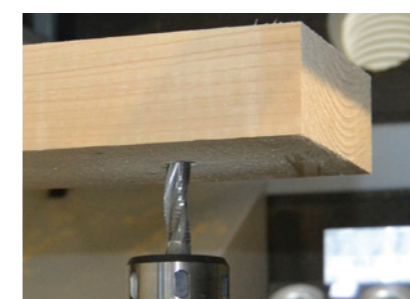
Mortise trimming with underfloor unit
