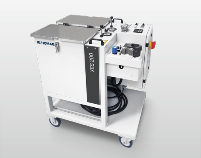
Service station ▪ Preheating and cleaning station for the QA65N application unit with one storage position ▪ High level of flexibility thanks to up to two vacuum containers for one QA65N application unit or one PUR melting unit with 2.5 kg/h capacity ▪ No vacuum pump and no nitrogen necessary ▪ With optional accessories also for application units for the powerEdge Pro/Pro Duo CNC edge banding unit
