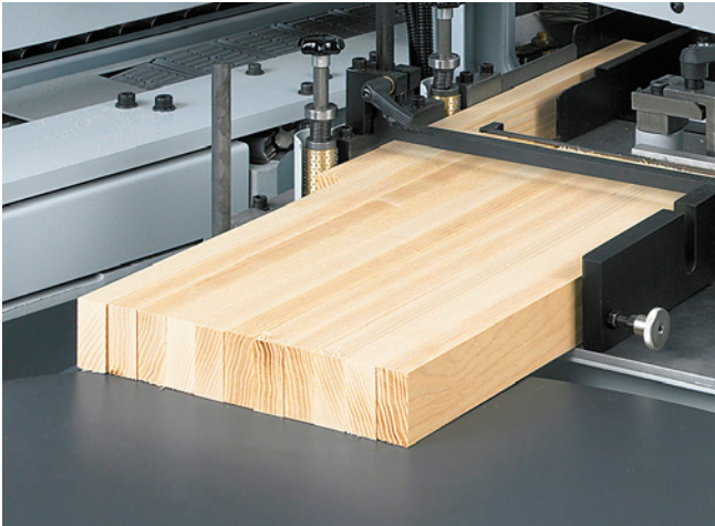
Processing of edges up to 20 mm For a high degree of flexibility in the edge selection, solid strips of up to 20 mm can be processed.
