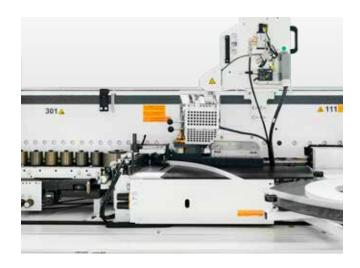
**Gluing unit:** Reliable hot melt glue application and perfect edge quality are provided by optimum combined workpiece preheating, Quickmelt application unit, pre-melting unit, magazine and pressure zone.
