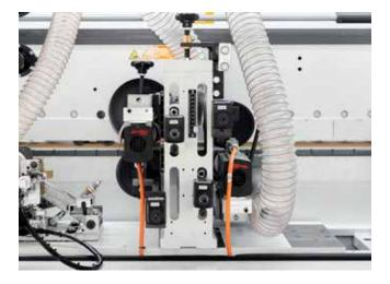
**Chamfer/radius trimming unit:** This 2-point adjustment trimming unit is ideal for rapid changes between thin and thick edges.
