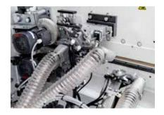
**Finishing units – perfectly coordinated:** The quality of the workpieces is increased by the profile scraper, the glue joint scraper, and the buffing unit.
