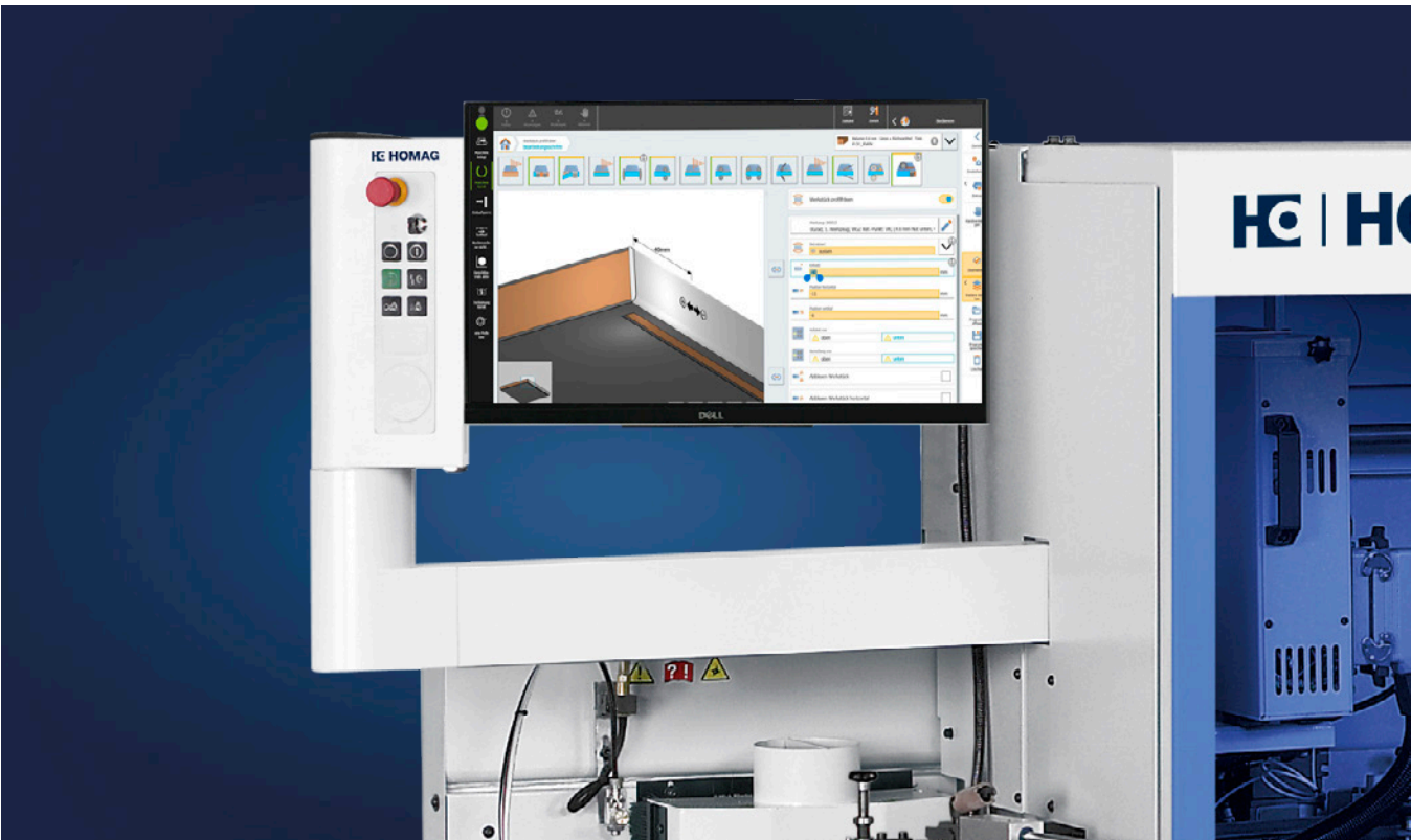
Intuitive operation with the powerTouch control system Control machine functions directly using the multi-touch, widescreen monitor. The ergonomic design, as well as numerous help and assistant functions, simplify operation significantly.
