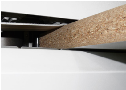
Belt-type top roll pressure Optional belt top roll pressure unit available instead of the standard roller top roll pressure unit.
