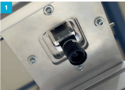
A camera system recognizes and checks the position of the connectors
