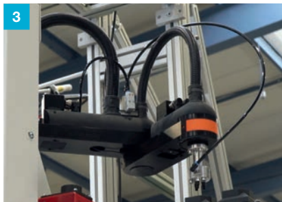
The robot separates the connectors and fills the magazines on the machine
