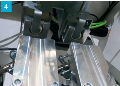
Transfer of the connectors to the hardware insertion unit
