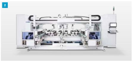
Batch size 1: Front processing with hardware inserting and robot handling
