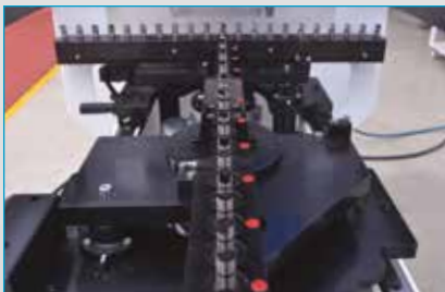
▪ Quick swivelling vertical drillblocks 0° - 90°
