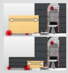
Control of the workpiece by sensor technology in X-direction. Depending on the workpiece dimensions the shortest distance to the next sensor is selected.
