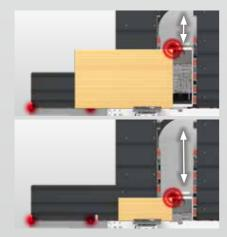
Control of the workpiece by sensor technology in Y-direction
