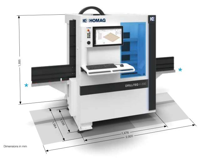
★ A corresponding safety distance must be maintained in the in and outfeed direction! (See documentation)
