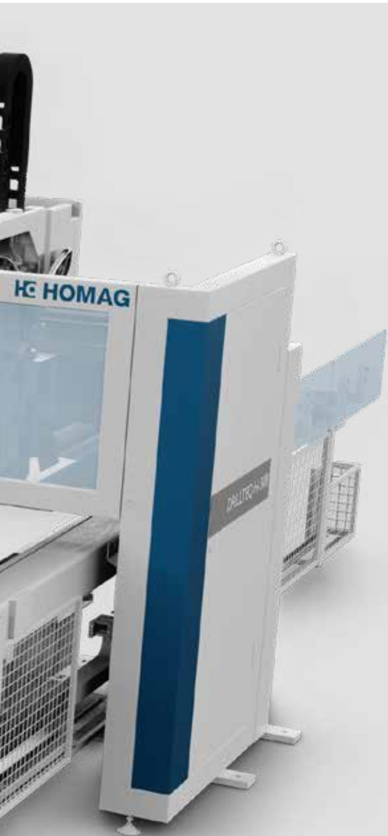
The lower safety fence prevents entry into the working area.
