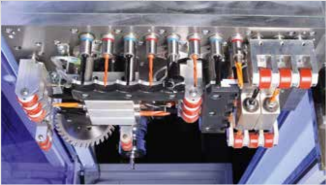
High-Speed Processing Unit | Top ▪ One Drilling Block V13, H6X, H6Y, optional routing spindle ▪ Two Drilling Blocks V13, H6X, H6Y, optional routing spindle ▪ High-Speed grooving saw unit in X direction
