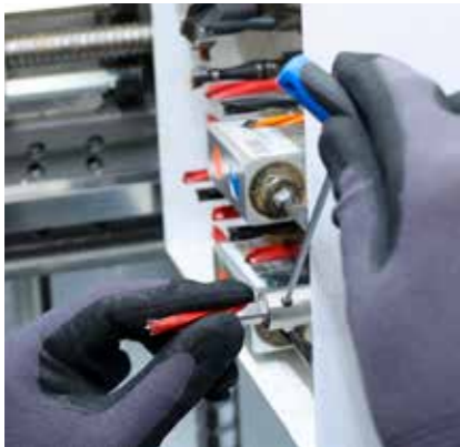
Weldon change system For a drill bit change with tools.
