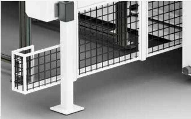
The lower safety fence prevents entry into the working area.
