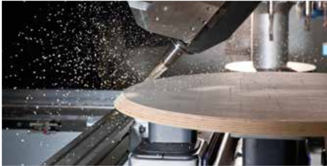
Chamfer cutting on a table top
