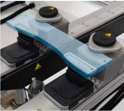
Multi-clamp for dual-circuit vacuum system. Vacuum-actuated clamping element for clamping strips and elements.
