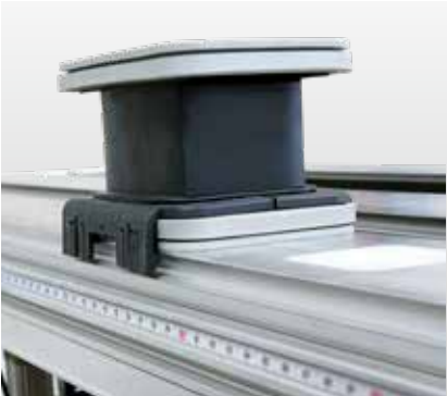
Measuring tape for positioning the suction units.
