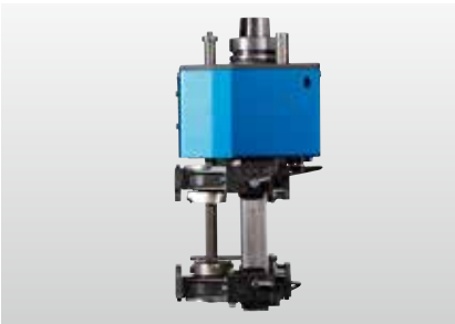
Combined flush trimming and scraper unit for flush trimming and scraper post-processing of the edge profile. The three-sided tracing of the unit balances out workpiece and edge tolerances and guarantees high processing quality incl. tools.
