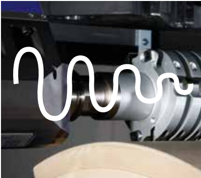
Liquid cooling and spindle sensor (optional for DRIVE5CS) – liquid-cooled routing spindles with hybrid storage offer a long service life. An additional vibration sensor detects tool unbalances and protects the spindle against overloading, due to high feed speeds for example.
