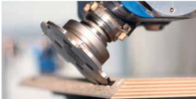
Cutting recesses for connecting fittings
