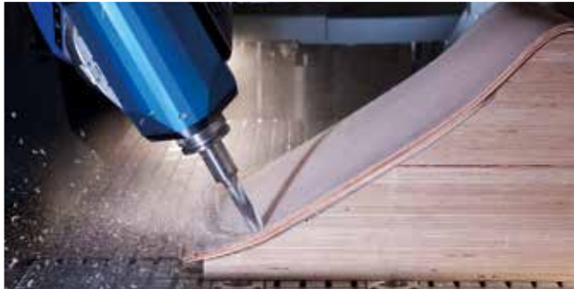
Routing of shaped wood
