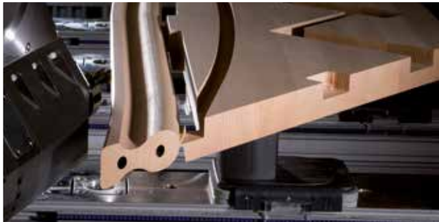
Holes for piling at narrow angles
