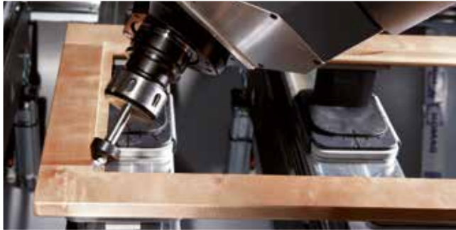
Square corner cutting for a glass rebate
