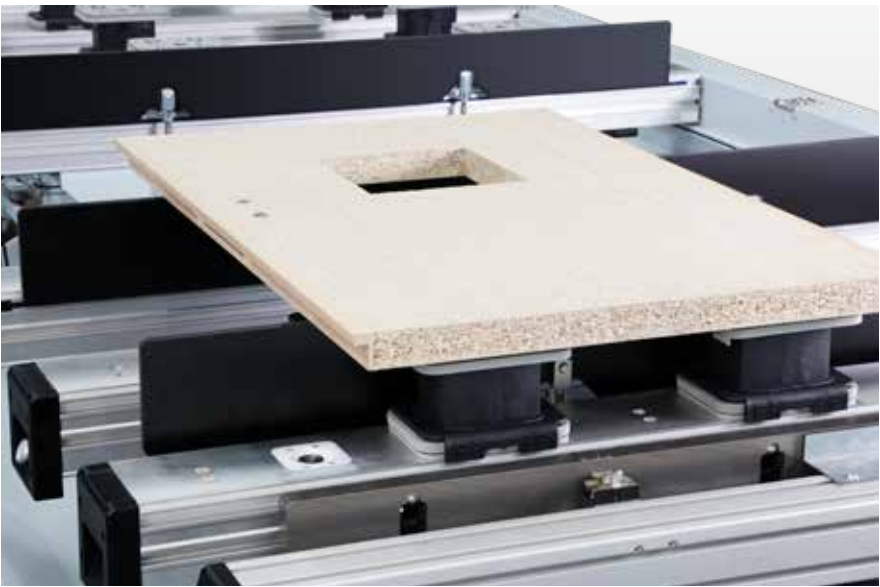
Workpiece feeding rail Solid feeding rails to ease placing of heavy workpieces with 2 pneumatic cylinders. Due to the linear movement of the feeding rails, the workpieces are not moved away from the stops during lowering, regardless of processing at the front or rear stops.
