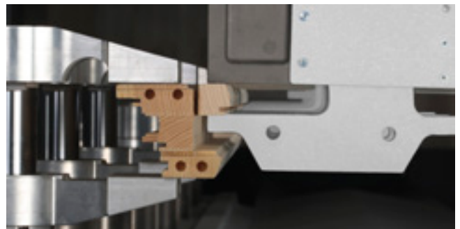
Extraction of glazing beads. Also allows a finishing cut of the glazing rebate. No addition processing required. Frame an glazing bead always stay together (Option)
