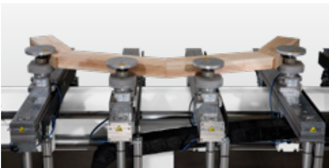
Processing of arches, doors and panels on a console table or automatically (option).
