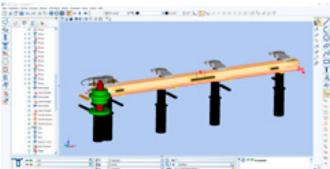
woodWOP programming system for single parts, ideal for the parametric manual programming of special parts and as an interface without the need for additional third-party software.
