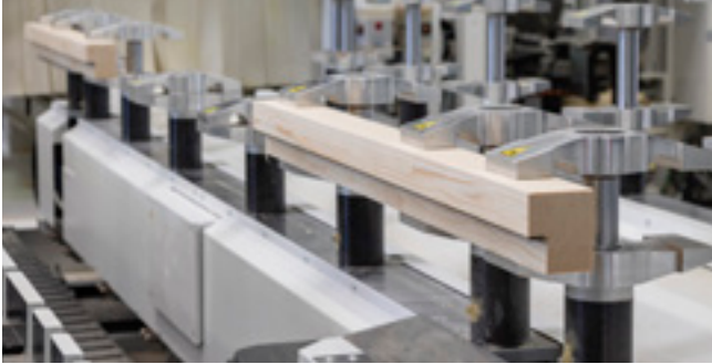
High performance thanks to clamping table with double assignment up to 1.9 m. Thus 2 parts in progress simultaneously
