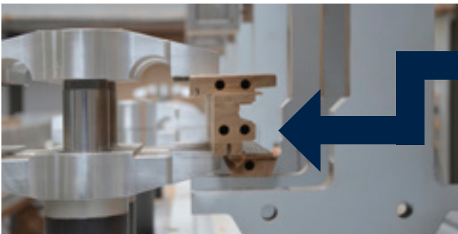
Maximum flexibility thanks to free clamping in all directions. With the ability to clamp in the rabbet for very narrow views CNC precision by gripper system with servo drives.
