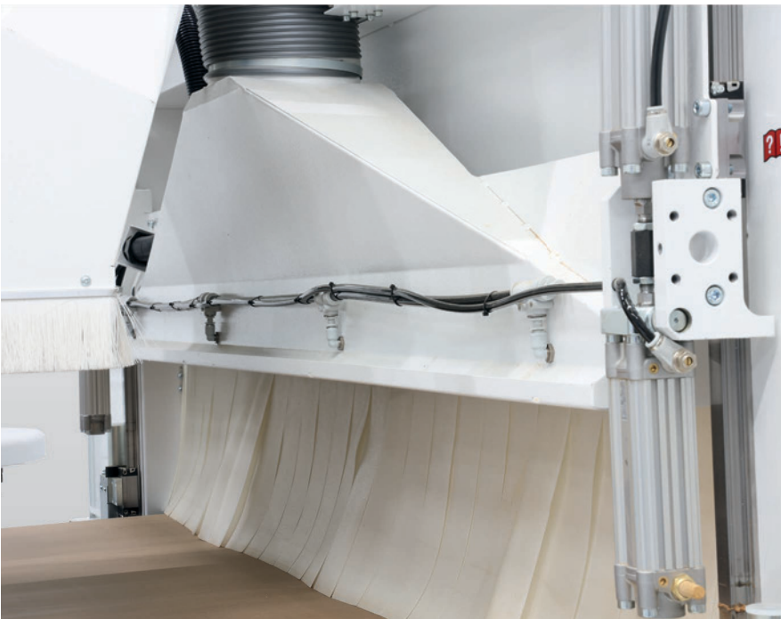
Suction at the end of the belt conveyor
