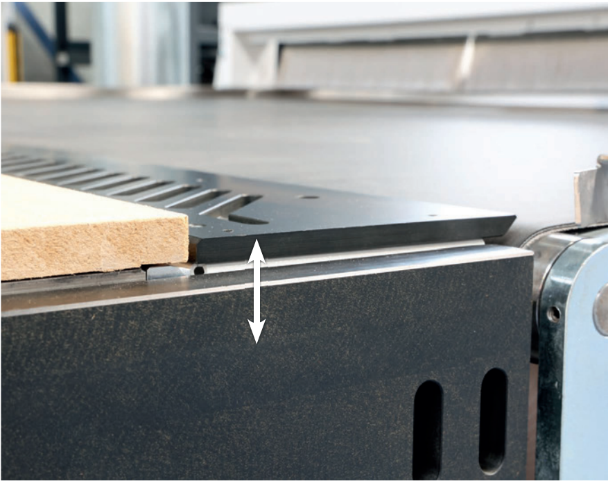
Suction from above the belt conveyor
