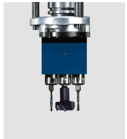
**Fitting drilling head**
