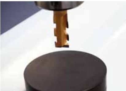
Tool length control After changing a tool, the length of the tool is queried and compared with the integrated tool databas
