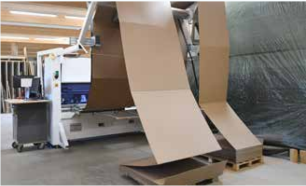
When using production lists , carton production is automated. Interruptions with individual cuts are possible without the last settings being "forgotten".
