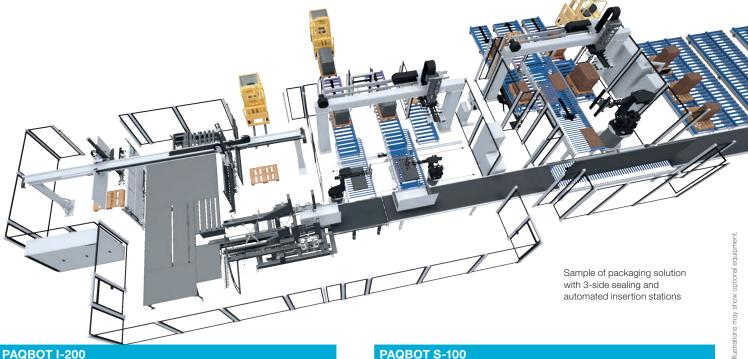
Automation for inserting workpieces, alternatively also a front edge protection, or a fitting box
