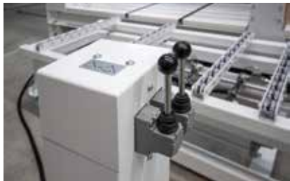
Operating the cabinet uprighter: By simply pulling on the lever, the cabinet uprighter aligns the pressed cabinet.
