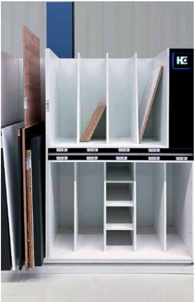
Offcuts with a system: The manual offcuts storage rack creates an overview and order, with maximized material use directly at the machine.
