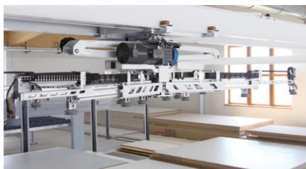
The highlight of the STORETEQ S-200 is its combination with suction traverse ST 71.
