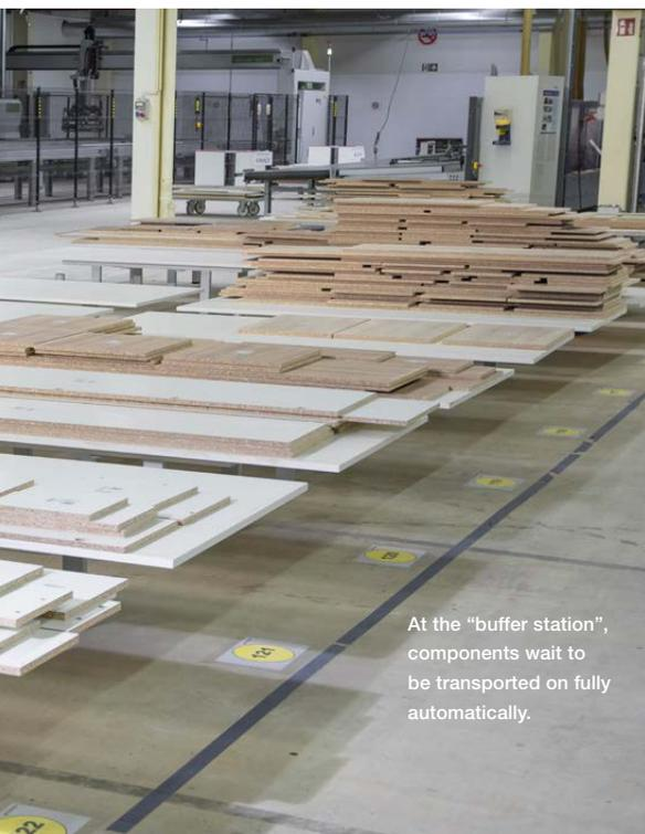
At the "buffer station", components wait to be transported on fully automatically.
