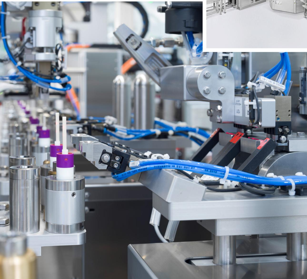
of Sales of Teamtechnik's medical technology business area in Freiberg am Neckar. The typical characteristic of this setup is a transport system that moves each workpiece in a circle from one workstation to the next – a proven method that enables high-quality mass production in a short time frame.
