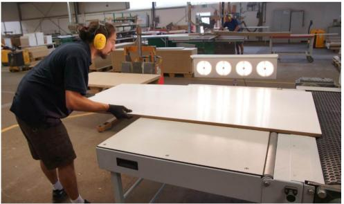
Picture 5 Control with inspection light after finish sanding
