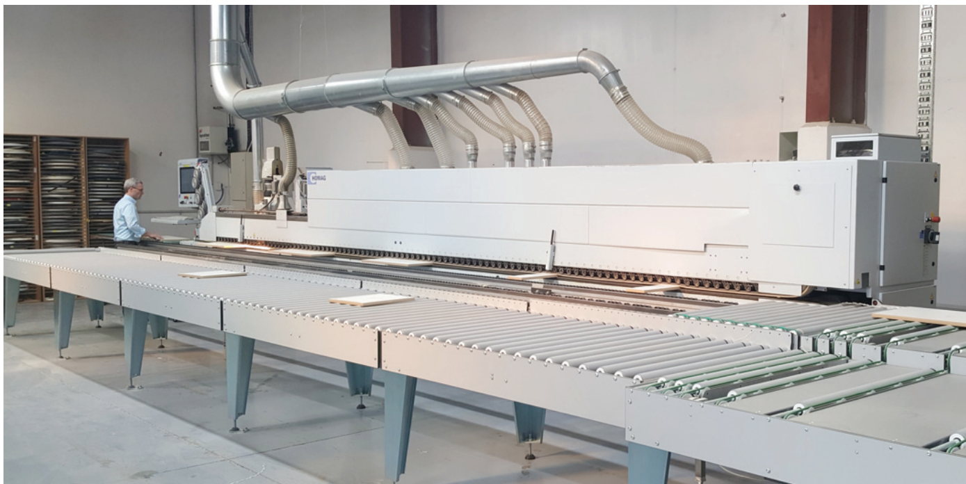
With their Homag KAL Panelform Industries have the option of three different adhesive types in the one machine: laser edge, PUR and EVA.
