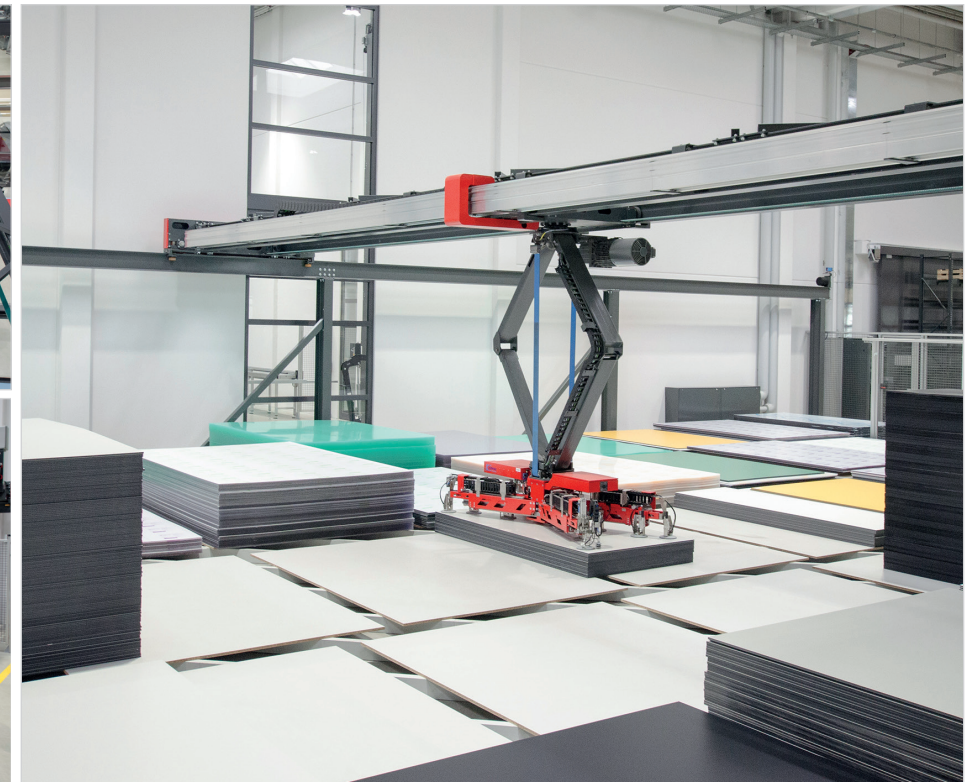
High stability of double scissors for exact panel handling
