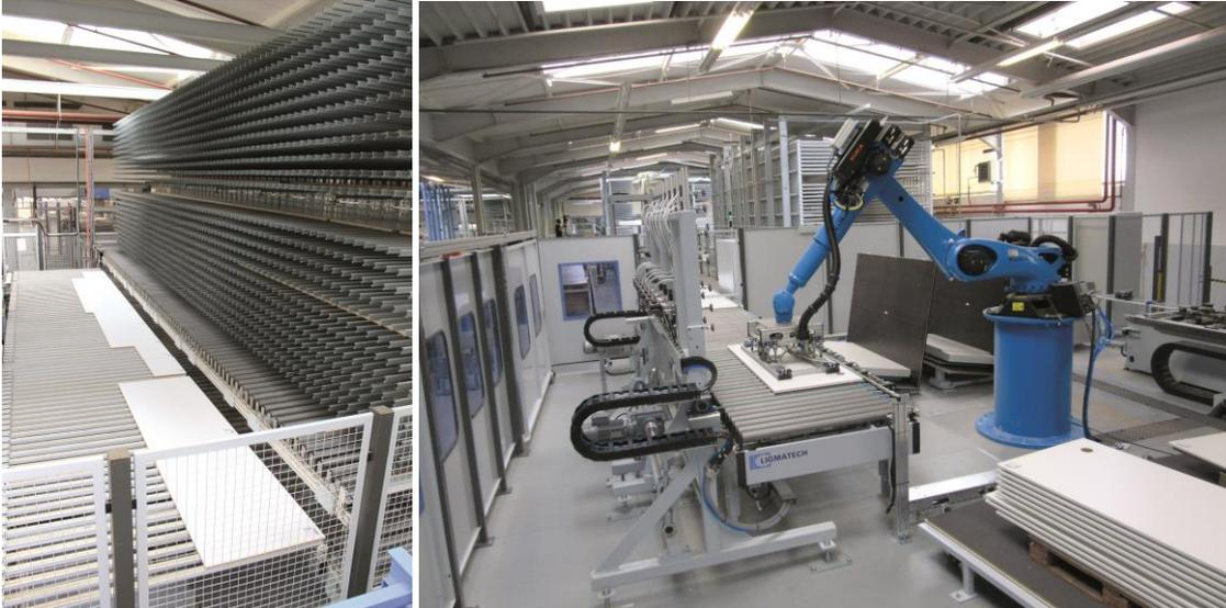
The robot cell is predominantly used for complex trimming and drilling tasks on table tops, taking the strain from the WEEKE drilling line.
