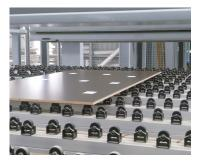
The Homag Automation TLF 211 board storage system at Kaiman Cabinets is coupled to a Holzma HPP 300 panel saw optioned to include the power concept and rear dedicated labelling station - every sheet in the stack can be labelled prior to cutting.
