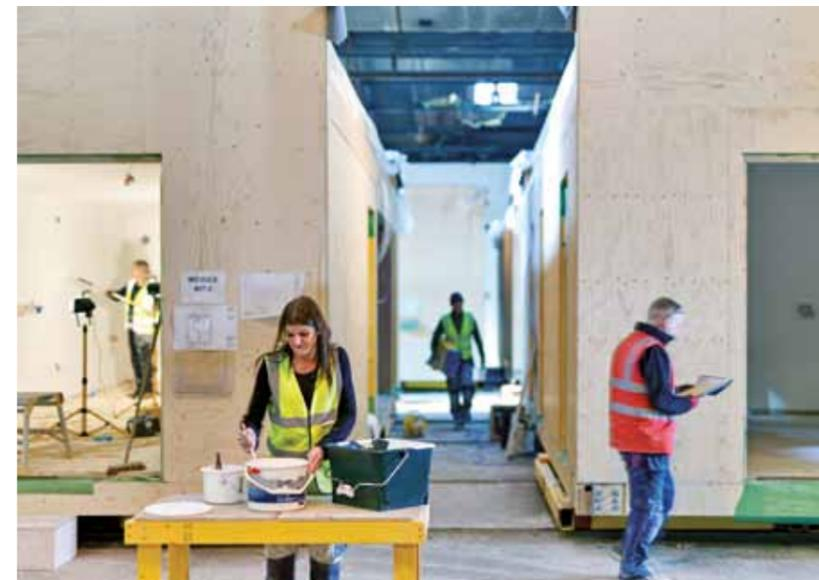
focused on building fully volumetric completed houses on a production line and the Herefordshire factory produces the timber-framed extensions.”
