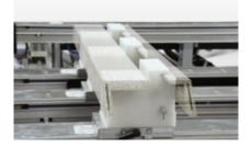
Clamping fixture for facings: Vacuum clamping fixture for a pair comprising rebate and ornamental facings according to customer design. Mounted on a base plate module.
