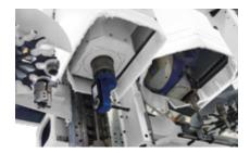
Rapid tool change: As it is designed with two trimming spindles, the chip-to-chip times are reduced and productivity is increased. While one spindle mills, the second inserts the tool for the next processing step.
