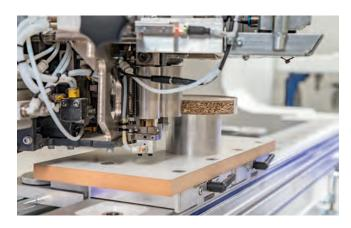
**Precise positioning:** Precise tracing and a feed roller with direct distance measurement guarantee CNC-accurate edge transport. This opens up new possibilities in the design of the shapes and allows perfect results for 360° gluing.
