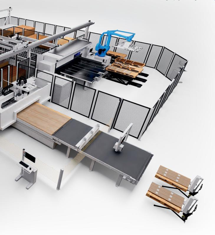
Combination: storage and saw. Standardized interfaces enable panel saws to be easily integrated in storage systems and instantly bring noticeable results as a production cell. The storage system puts panels into or removes them from storage quickly, fully automatically and accurately, picks them or transports them to the connected saw. The storage-saw combinations cover the logistical requirements – from woodworking shop customers through to industrial furniture makers.
