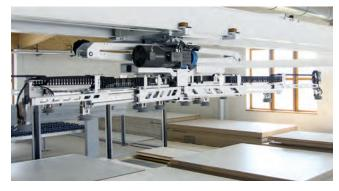
The **ST71 suction traverse** in X geometry is the ideal optional feature for the panel storage. The self-learning cross rail generates the data required for panel handling independently and thus ensures dependable process reliability. The operator does not have to enter anything.
