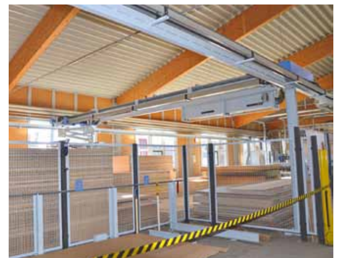
The automatic plane storage system TLF 211 can accommodate and manage all panels up to the biggest standard format 5 600 x 2 200 mm.
