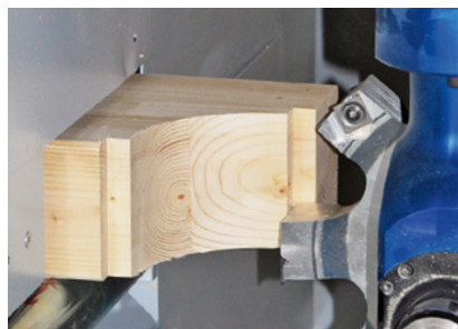
Rafter head processing
