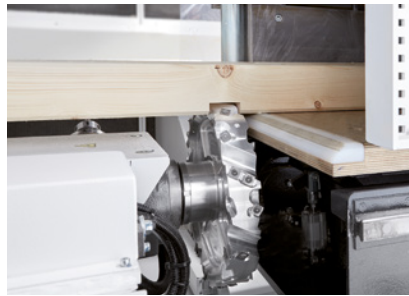
Lap joint with side milling cutter
