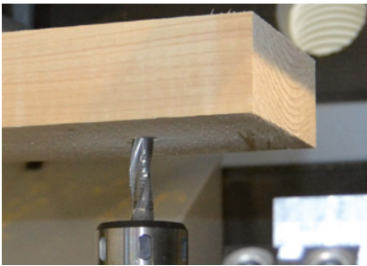
Mortise trimming with underfloor unit
