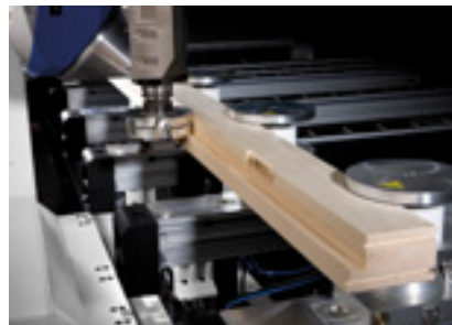
Profiling of frame components
