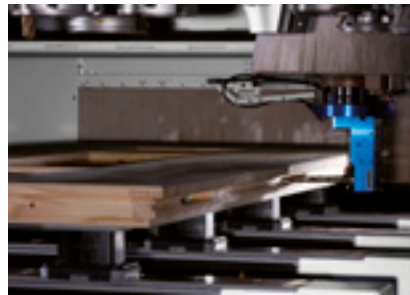
Lock case trimming on front doors
