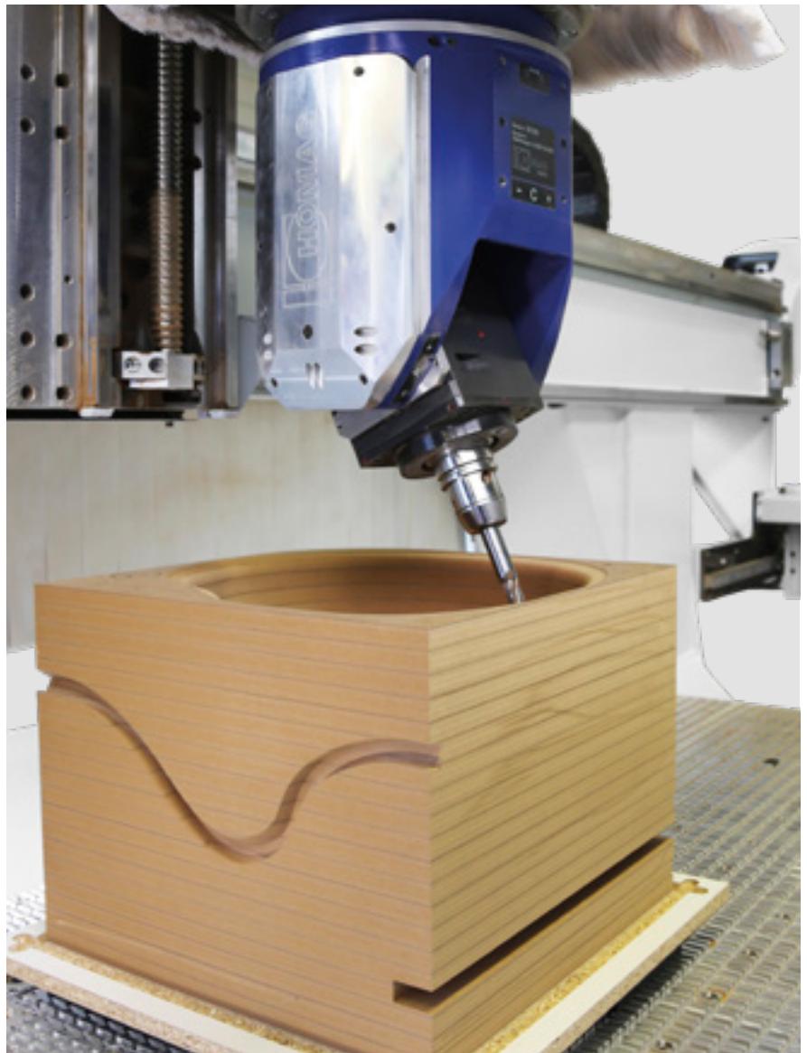
Trimming of components with large Z height
