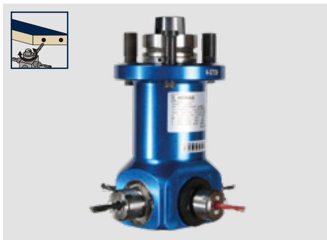
2+2-spindle drilling/trimming unit: The 4-sided spindle outlet makes available four different drilling and trimming tools without tool change. Continuous shaft for greater rigidity and processing without change of direction when using clockwise and counterclockwise rotating tools, e.g. when trimming out recesses for door hinges.
