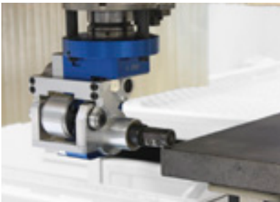
Traced flush trimming of overhanging edges on postforming profiles
