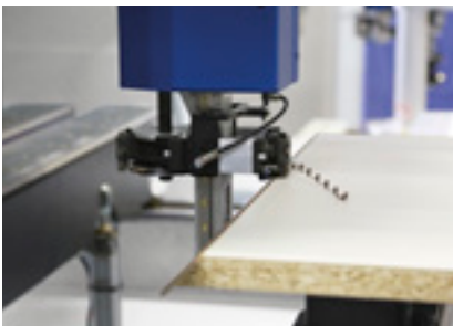
Scraping of mitered edges
